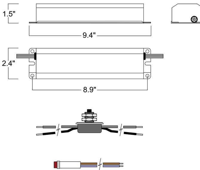
A separate test switch and charging indicator light are provided.
